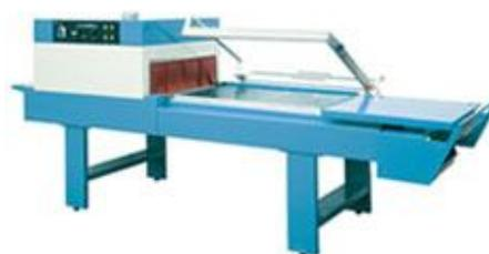
*These systems have been conceived to be used in case more automation is required, in fact the only thing the operator has just to do is to insert the product into the film and to move it onto the sealing area, as the rest of the working cycle (sealing, product removal and transfer inside the shrink tunnel) happens automatically.*
